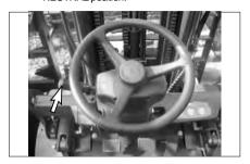
Engage the parking brake, if not already engaged. Place the transmission directional control lever in the NEUTRAL position.
