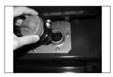
Raise the hood and seat assembly. Loosen the bolts of the hydraulic tank cover, and remove the hydraulic tank cover with filter assembly.
