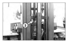
7. In case of Full Free Lift Mast, extend the primary cylinder to full length and then check the clearance and over lapped dimension between carriage stopper bolt or block (1) and Inner mast stopper block (2). Adjust the chain anchor bolt (3) so that clearance should be 14 ± 2 mm.
