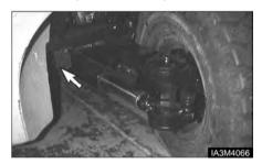
Inspect the suspension mounting bolts. Tighten suspension mounting bolts, if necessary, to 240±30 N·m (180±20 lb·ft).
