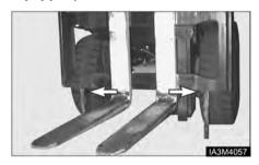
Raise the carriage high enough to gain access to the side thrust rollers on the back side of the carriage. Block the carriage in this position.
