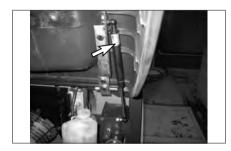
The hood and seat assembly is held up by a support cylinder. Make certain the air cylinder is operating properly and securely holds the hood up before doing anything in the engine compartment.
