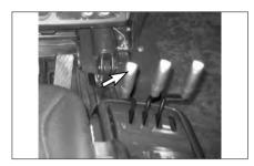
NOTE: To prevent a sudden change of position of the load, operate all lift, tilt and attachment controls smoothly.
