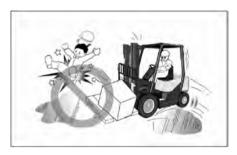
Do not drive on slippery surfaces. Sand, gravel, ice or mud can cause a tipover. If unavoidable, slow down.
