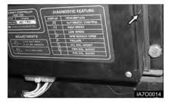
ASC-205 has internal indicator on the right side of the controller for displaying the selected gear and the abnormal condition.
