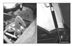
Lightly oil the hood latch mechanism and the rod for the hood support cylinder.
