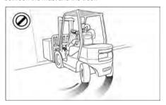
Do not start, stop, turn or change direction suddenly or at high speed. Sudden movement can cause the lift truck to tip over. Slow the speed of your truck and use the horn near comers, exits, entrances, and near people.
