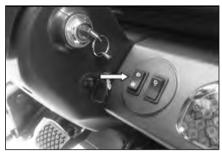
This switch initiates regular regeneration process of the post-treatment device.
