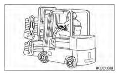
Tilt elevated load forward only when directly over unloading area and with load as low as possible.
