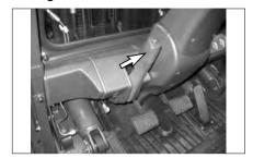
Pull the lever BACK to engage the parking brake.
