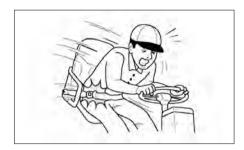
In the event of a tipover, the seat and restraint system should be inspected for damage and replaced, if necessary.
