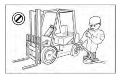
Forklift trucks may only be refueled at specially reserved locations. Switch off the engine when refueling. Smoking and handling of naked flames during refueling are strictly prohibited.
