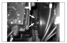
1. Inspect for loose retaining bolts. Check for worn or damaged bearings.
