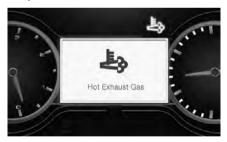
Display that notifies the operator of automatic SCR cleaning
