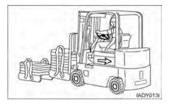
Use special care when operation on grades. Do not angle across or turn on grades. Do not use lift truck on slippery grades. Travel with forks downgrade when unloaded. Travel with load uporade.
