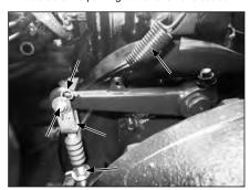
Make sure the parking brake is secured by the stop pin. 6. Remove the pin and cotter pin. Tighten the nut to more compress the spring, and pull down the Ushaped linkage while turning it. And then reinstall the pin and cotter pin, and return the nut to the Ushaped linkage.
