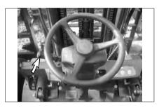
Select the direction of travel by pushing the directional lever FORWARD for forward direction or by pulling the lever BACK for reverse direction.
