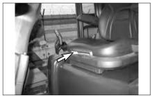
**15.** To position the seat, PUSH the lever away from the seat track and move the seat forward or backward to a comfortable position.
