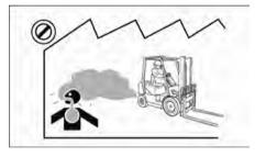
Exhaust from all internal combustion engines contains carbon monoxide, a colorless, odorless, tasteless, poisonous gas. Exposure to carbon monoxide can cause serious injury or health problems, including death, and avoid unnecessary idling of the engine. If nausea, dizziness or headaches are experienced stop the truck and seek fresh air.
