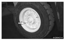
Install steer wheel. Put two nuts opposite (180°) each other. Tighten both. Install remaining nuts. Tighten all nuts in a sequence opposite (180°) each other. Tighten to 440+35 N-m (325+25 lb-ft).
