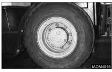
Install drive wheel. Put two nuts opposite (180°) each other. Tighten both.
