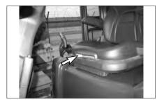
Check the operation of the seat adjuster rod. Make sure that the seat slides freely on its track. Lightly oil the seat slider tracks if necessary.
