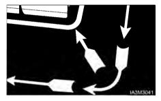
In narrow aisles, keep away from the stockpile when turning into the aisle. Allow for counterweight swing.
