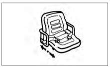
Adjust the seat before operating the lift truck. After adjusting, set the seat to make sure it is properly locked. Do not adjust the seat while the truck is in motion.
