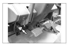
Push the lever down to raise the hood and seat assembly. Make certain the support cylinder will hold the hood open.
