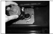
Stop the engine and check the oil level. With all cylinders retracted, maintain the oil level to the FULL mark on the dipstick.
